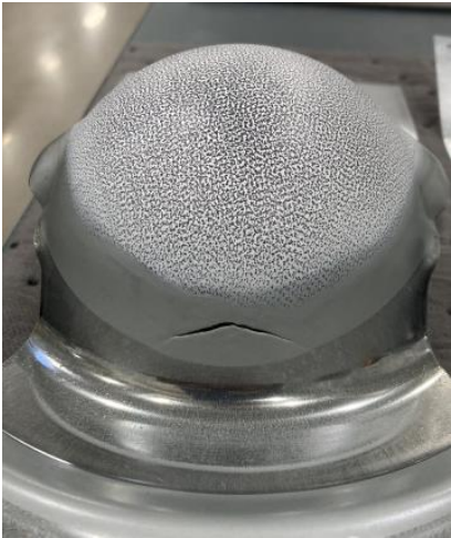
Test sample with DIC speckle pattern
