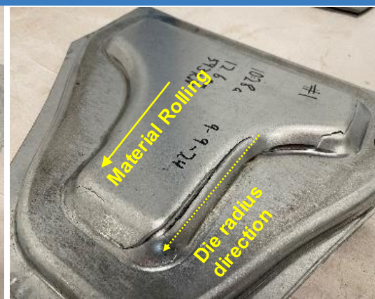
Fracture specimen with rolling parallel to die radius direction
