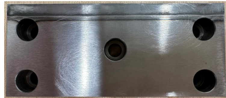
Laser hardened 4140 (machined from prehard bar stock) Trim Tool
