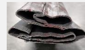
→ Test vs CAE Cross Section View
