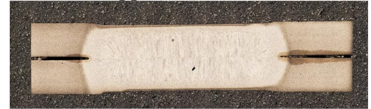
3G-1180 Optimized Spot Weld (Nugget size of 7 mm)
