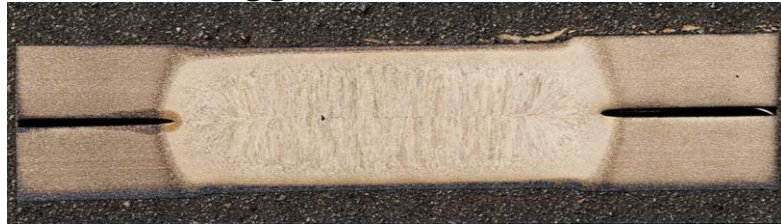
3G-980 Optimized Spot Weld (Nugget size of 7 mm)
