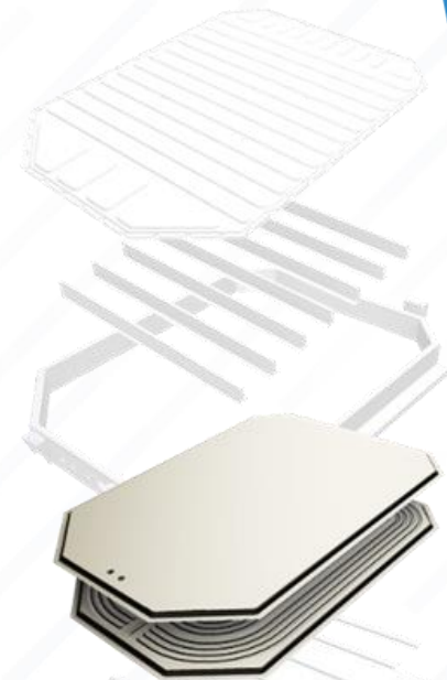
Cooling system made of CR Steel – 0.6mm
