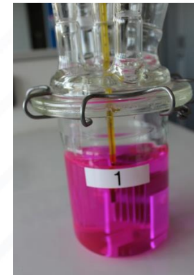
Coolant reactor (V = 750 ml)
