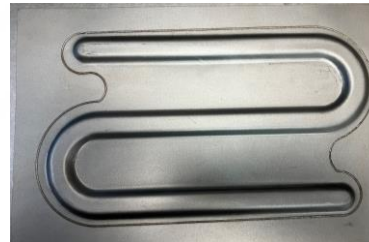
Physical part - “S – shape” laser welded
