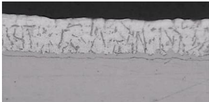
Scanning electron micrograph of Alusi® (AS) for cold-stamping cross-cut
