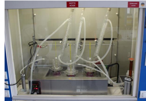
Equipment with 3 thermostated reactors
