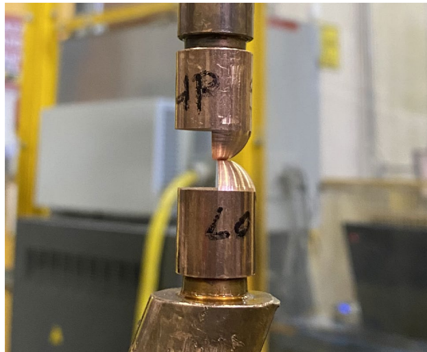
Half-sectioned 6R50 electrode
