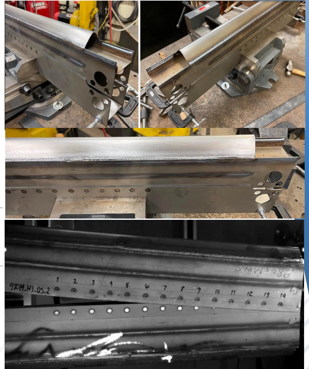
Caiman Mode-III (shear-dominated load)
