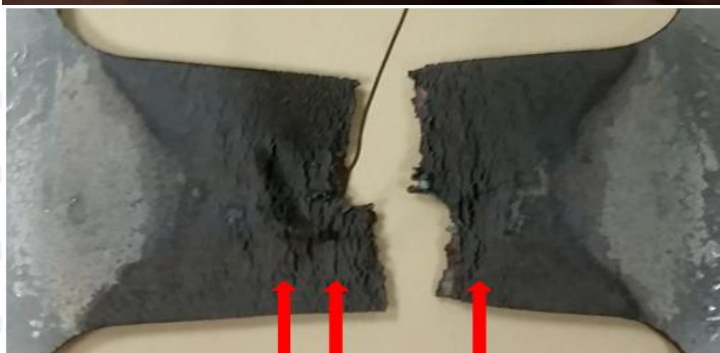
Liquid Metal Embrittlement Cracks
