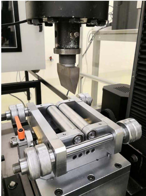
3-point bending fixture (VDA 238-100)
