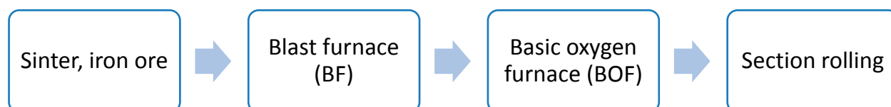
Figure 3-3: Structural section BF/BOF process flow
